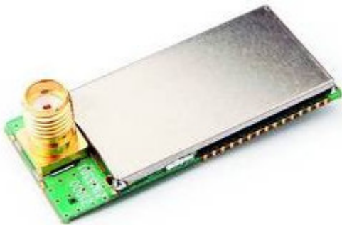
Jennic Microcontroller with Sedona and Antenna
